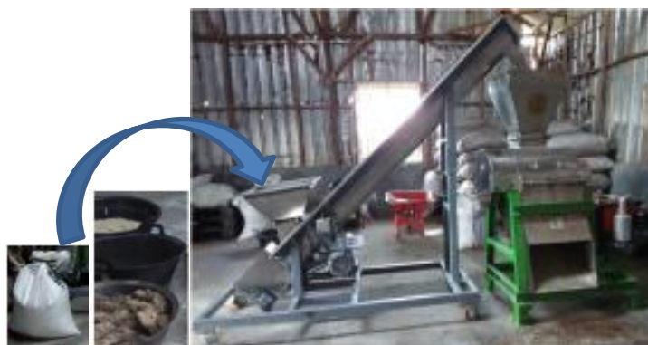
Gambar 36. Uji kinerja lapang screw conveyor
