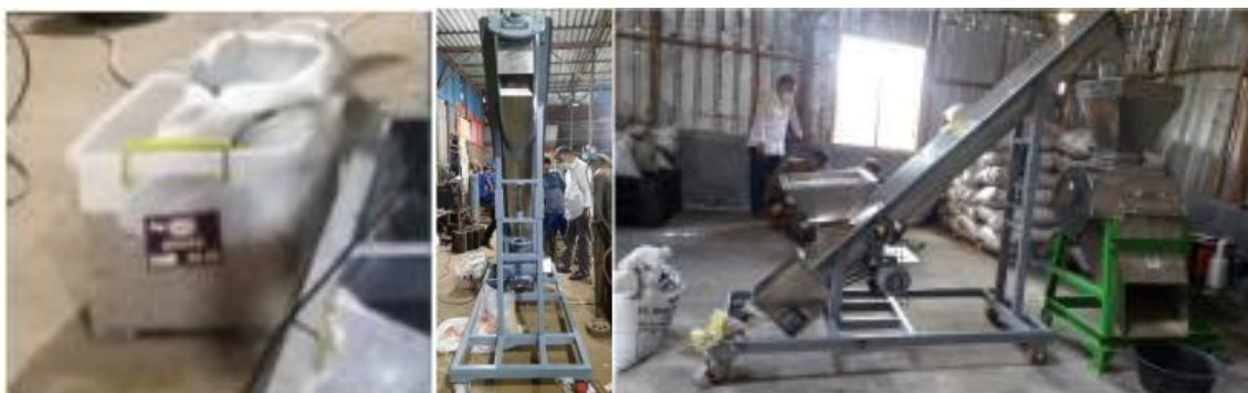
Gambar 32. Uji fungsional screw conveyor
